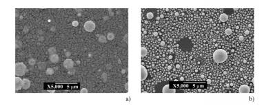
Figure 2. Pb thin film deposited at room temperature a) and at about 200° C b) of substrate temperature.
