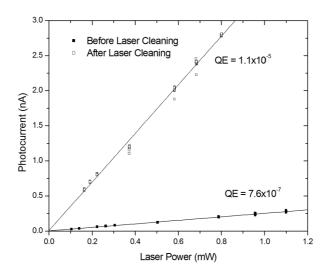
Figure 1. Photocurrent of Y photocathode as a function of laser power before and after in-situ laser cleaning treatment with photons at 406 nm.
