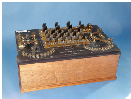
Ponte di Wheatstone (University of Nebraska, Lincoln, USA).
