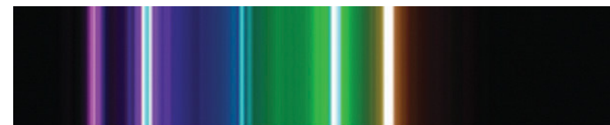
Hg vapor spectrum (350-700 nm)
