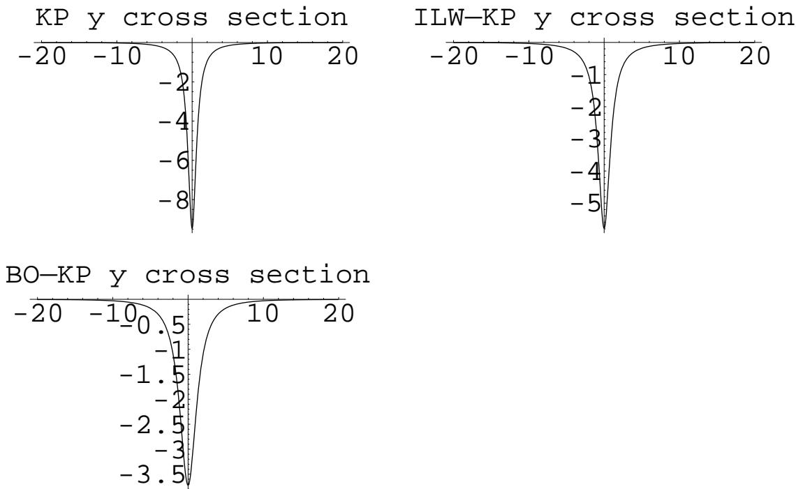
Figure 5:  $y$  cross sections  $w(0, y)$   $\delta = 1; \alpha = 1/10$ ,  $\delta = 10; \alpha = 1$ , and  $\delta = 100; \alpha = 10$ , i.e. the KP, ILW-KP, and BO-KP regimes, respectively. In each case, the  $x$ -dir. speed  $c = -1$ .
