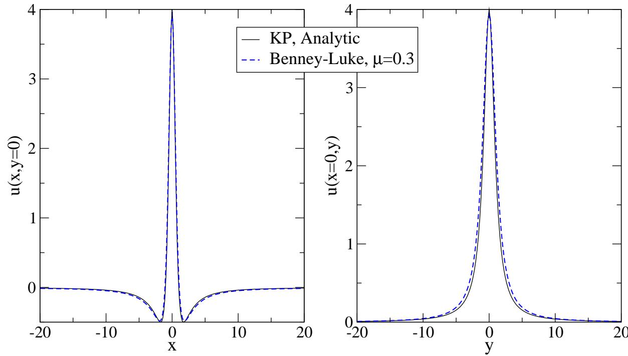
Figure 1: Wave profiles for the KP and BL eq.
