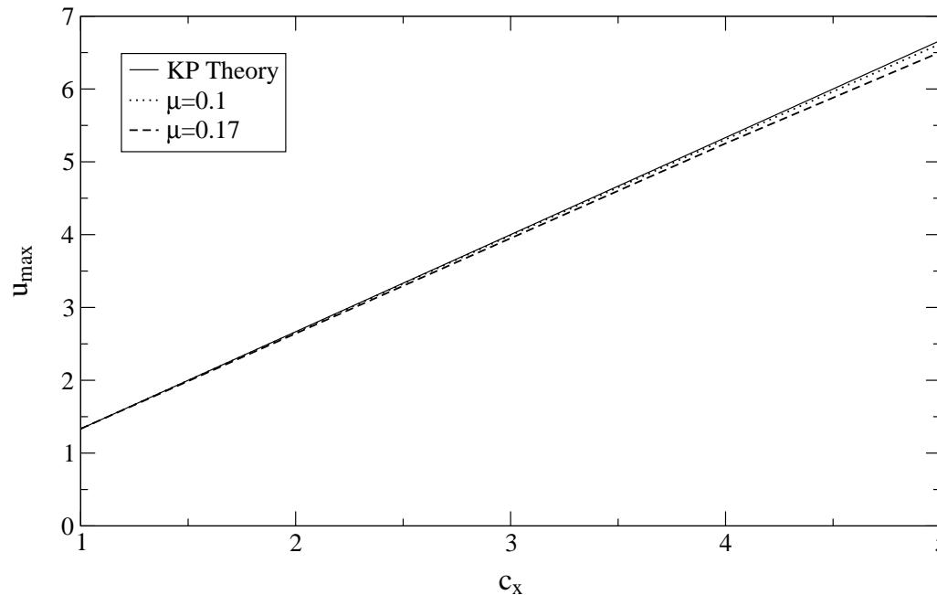
Figure 7:  $u_{max}$  vs.  $c_x$  the full WW equations for various values of  $\mu$ . Fig. also shows that the Benney-Luke/KP equations are good approximations to full WW eq. in this range of parameters.
