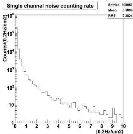
Figure 2. Distribution of RPC single channel counting rate for a high voltage of 9600 V and nominal voltage front-end threshold ( $T=20$  °C and  $P= 980$  mbar).
