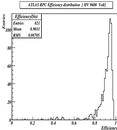
Figure 1. Distribution of the RPC average readout strip panel average detection efficiency for a high voltage of 9600 V and nominal voltage front-end threshold ( $T=20$  °C and  $P= 980$  mbar).
