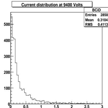
Figure 3. Gap current distribution for RPC ATLAS chamber for a high voltage of 9400 V
