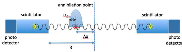
Figure 2. The TOF concept. Annihilation point localization along the coincidence path between the two scintillators is improved by measurement of the time difference  $\Delta t$  between the two signals.
