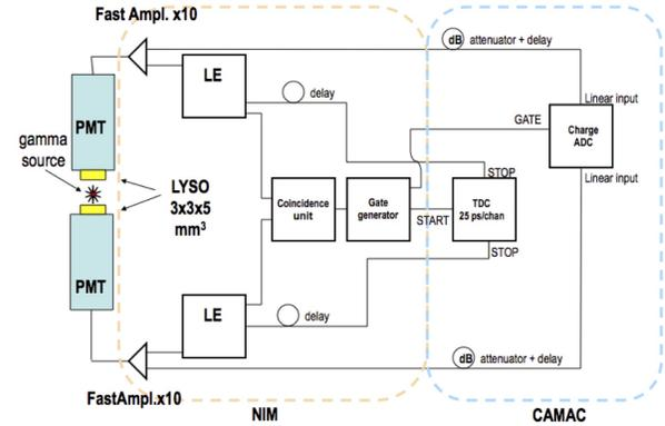
Figure 3. Signal processing for high resolution timing measurement with  $^{22}\text{Na}$  gamma source.
