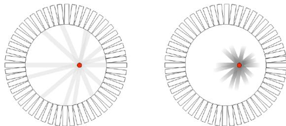
Figure 1. The PET concept. Localization of  $e^+e^-$  annihilation point is obtained by intersecting the back-projection lines between two opposite scintillators measured in coincidence [1].
