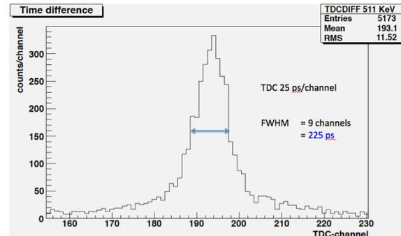
Figure 4. TOF measured for 511 keV  $\gamma-\gamma$  correlated events from  $^{22}\text{Na}$   $e^+e^-$  annihilation. LYSO  $3\times 3\times 5$  mm<sup>3</sup> polished crystals were directly coupled from one 5 mm long face to Hamamatsu R9880U110 PMTs. Other faces were wrapped in teflon.
