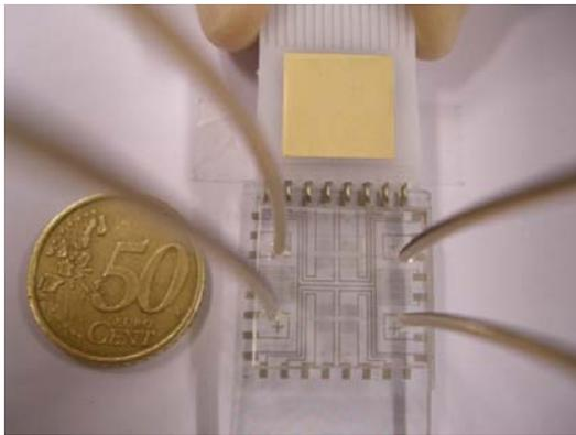
**Figure 1.** Biochip layout with interdigitated electrodes, temperature sensors and heaters, PDMS microfluidic components (chambers with microchannels), inlet and outlet tubes.
