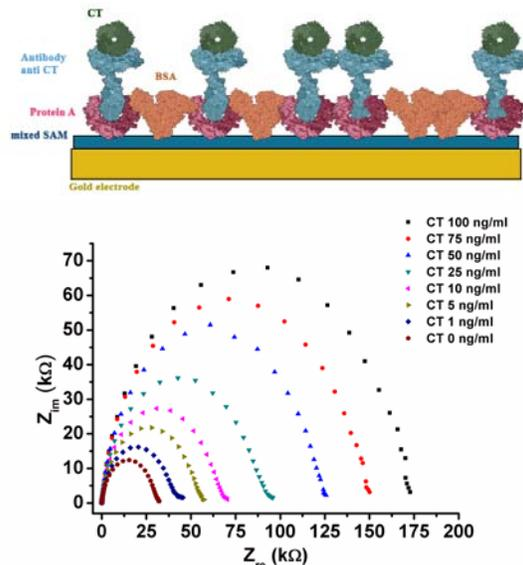
**Figure 2.** (top) Schematic representation of electrode functionalization. (bottom) Nyquist spectra at decreasing CT concentrations.
