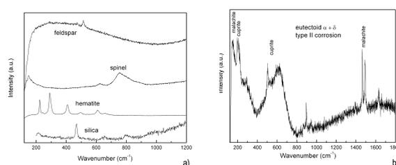
Figure 2. Typical micro-Raman spectra of the coin: a) before laser irradiations in four different areas and b) after laser irradiations.
