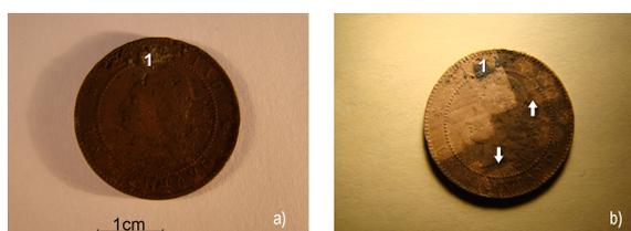
Figure 1. The Argentinean coin a) before and b) after laser cleaning treatments.
