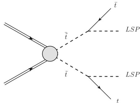
Figure 1. Diagram of pair production of stops with subsequent decay with 100% branching ratio to a top quark and the LSP (Neutralino).
