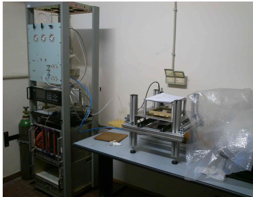
Figure 1. The laboratory set-up for testing a prototype of triple GEM with cosmics and sources (right table) and development of the gas distribution and control system for the JLab12 front tracker GEM chambers (left rack).
