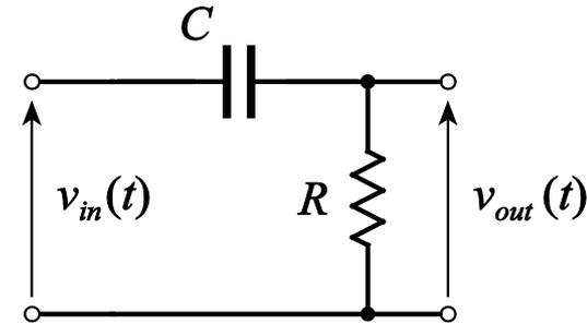
$$\bar{V}_{out}(\omega) = \bar{V}_{in}(\omega) \frac{R}{R + \frac{1}{j\omega C}} = \bar{V}_{in}(\omega) \frac{j\omega RC}{1 + j\omega RC} = \bar{V}_{in}(\omega) \frac{j\omega\tau}{1 + j\omega\tau},$$
