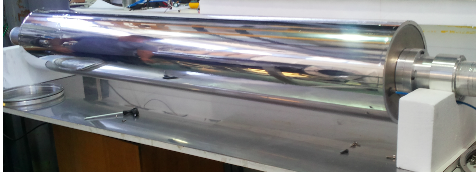
Figure 4.12: Prototype of mylar inner foil.
