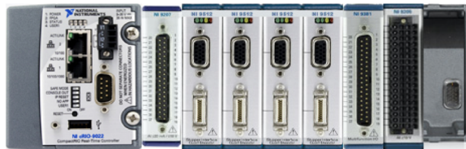
Figure 5.26: cRIO Controller with chassis and modules.
