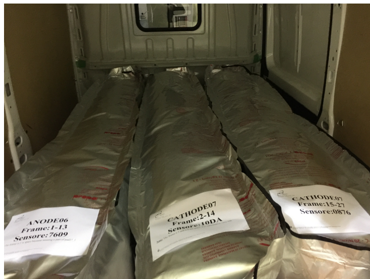
Figure 6.15: The frames are wrapped in a welded seal bag.
