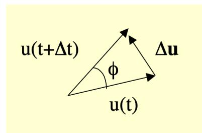
$$\frac{|\Delta \hat{u}|}{\Delta t} = \frac{|\Delta \hat{u}|}{\Delta \phi} \frac{\Delta \phi}{\Delta t} = \frac{|\hat{u}| \sin(\Delta \phi)}{\Delta \phi} \frac{\Delta \phi}{\Delta t} = \frac{\sin(\Delta \phi)}{\Delta \phi} \frac{\Delta \phi}{\Delta t}$$
