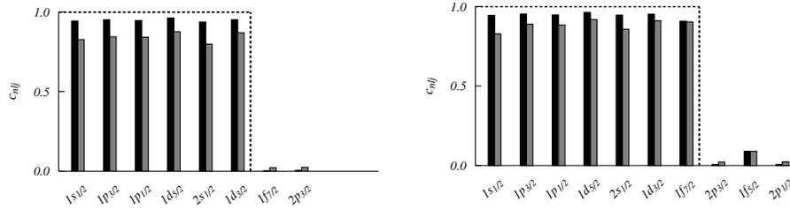
Figure 9.3: Comparison between the occupation numbers of an IPM, dashed lines and those of natural orbits indicated by the histograms. These latter numbers are calculated by using two different correlation functions. The system under investigation is the  $^{48}\text{Ca}$  nucleus. The figure on the left hand side indicates the results for the protons, the figure on the right hand side that for the neutrons.
