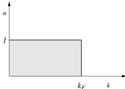
Figure 17.1: Distribution function  $n(k)$  for the Fermi gas ground state.
