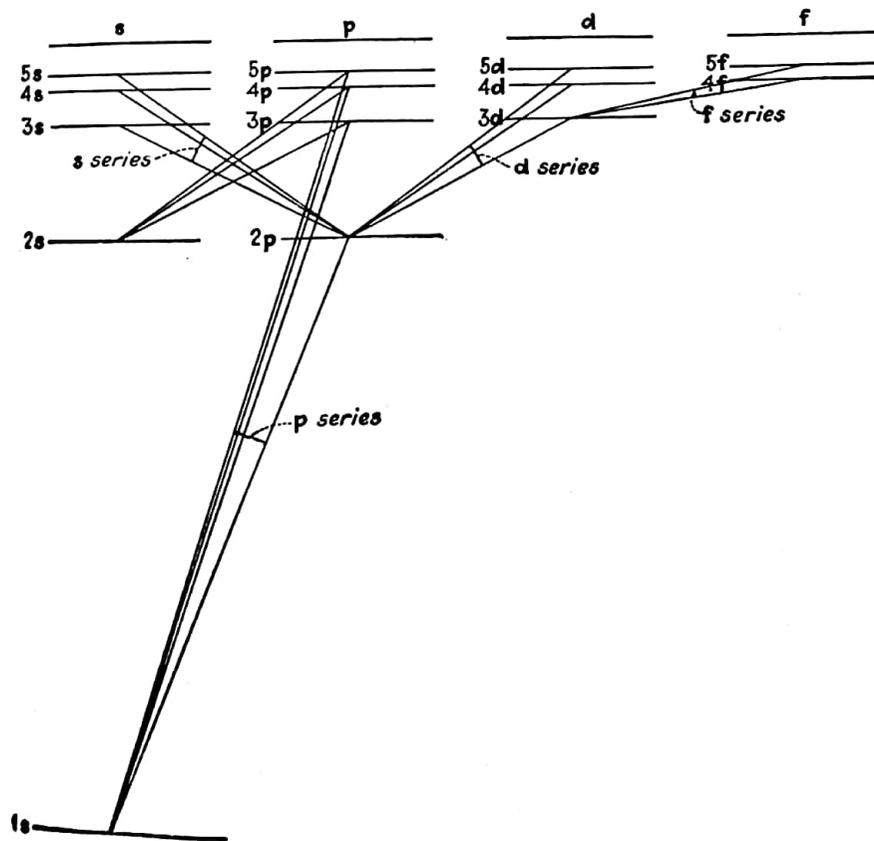
Fig. 5.4.1. Energy levels and allowed transitions and series in hydrogen.
