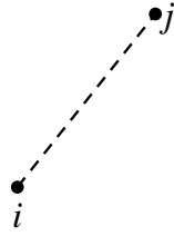
Figure 2.1: Graphical representation of the second term of eq.(2.14). The dashed line represents the correlation function h . The black dots represents the integration points i and j .
