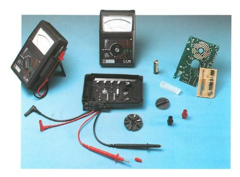
**The shockproof case.** An accessory recommended for the whole C.A 400 series. The prods can be stored on the side of the case when not in use.
