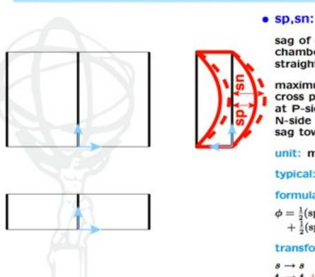
sag of cross plates out of chamber plane, tubes remain straight
