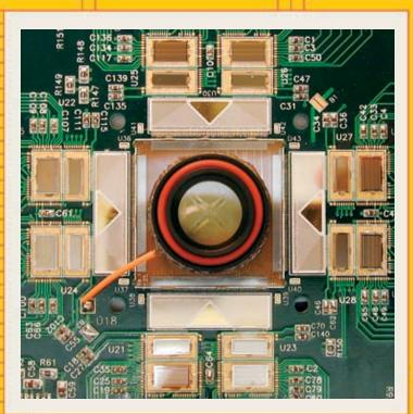
In the center of this chip, an array of 512 electrodes no bigger than the head of a pin records signals from neurons that transmit information from the retina.
