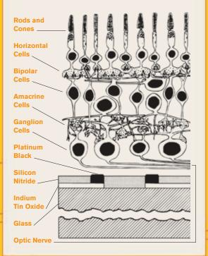
A computer-generated pattern of light is focused on the retina. The electrode array below senses the retina's response so scientists can understand the conversion of light to electrical signals.
