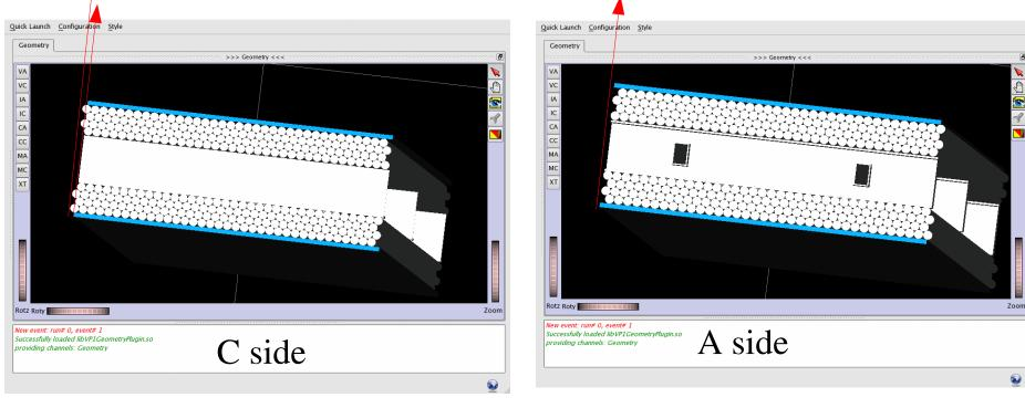
Right-arrow(C-side): MuonGeoModel-00-05-29 recover the ~10microns disagreements wrt Amdc when A-lines are applied
