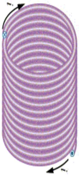
$$\oint_{\Gamma} \vec{B} \cdot d\vec{l} = \mu_0 \sum i_c \Rightarrow \int_a^b \vec{B} \cdot d\vec{l} + \int_b^c \vec{B} \cdot d\vec{l} + \int_c^d \vec{B} \cdot d\vec{l} + \int_d^a \vec{B} \cdot d\vec{l} = \mu_0 \sum i_c$$
