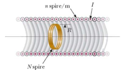
$I_{sol} [Ampere] = (0.5t)$ ,  $B = \mu_0 n I$ ,  $\epsilon_{ind} = -\mu_0 n \times 0.5 \times N \pi R^2$ ,  $i_{ind} = -\mu_0 n \times 0.5 \times N \pi R^2 / 100\Omega = 4.8\mu A$
